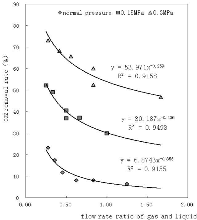
Fig. (2).  $CO_2$  removal rate changing under different scrubbing pressure condition.
